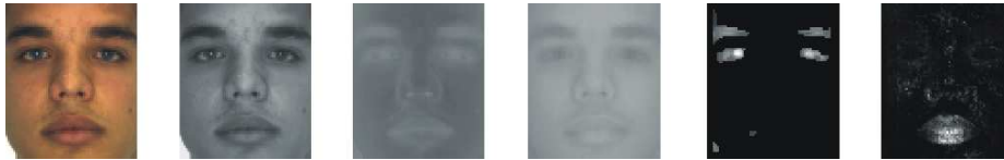
Fig. 1. From the left: face image (M_023_1 from the AR database), Y , C_b and C_r channels, eye map and mouth map.
